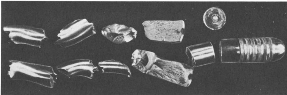
Fig. 161. Piston broken at pressure of 18,000 atm.
